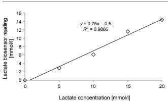
**Fig. 1.** The linearity of the lactate standard solution measured with the lactate biosensor at a temperature of 30°C
