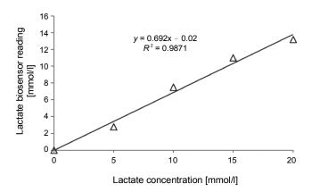
**Fig. 3.** The linearity of the lactate standard solution measured with the lactate biosensor at a temperature of 55 °C
