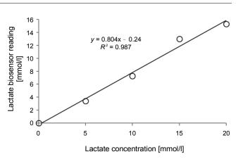
**Fig. 2.** The linearity of the lactate standard solution measured with the lactate biosensor at a temperature of 45°C
