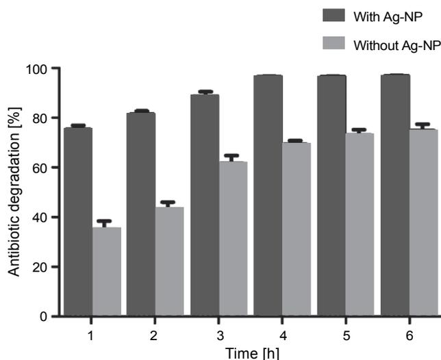
Fig. 5. Effect of contact time on ampicillin degradation
