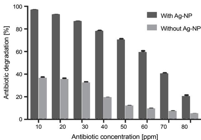
Fig. 6. Effect of initial ampicillin concentration on degradation
