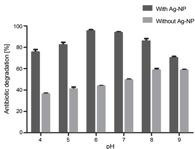
Fig. 8. Effect of pH on the photocatalytic degradation of antibiotics
