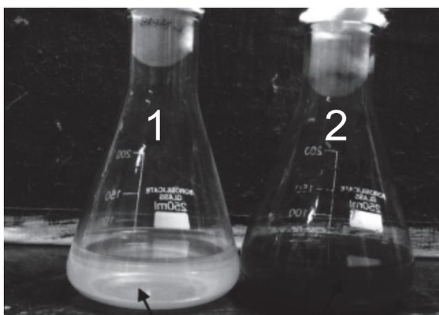
Fig. 1. The synthesis of AgNPs by *Pleurotus ostreatus* resulting in a change of the color of the suspension 1) before and 2) after synthesis
