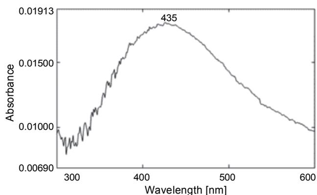
Fig. 2. UV-visible absorption spectra of Ag-NPs
