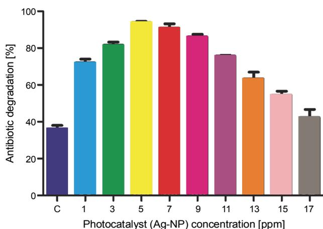
Fig. 7. Effect of photocatalyst concentration on antibiotic degradation
