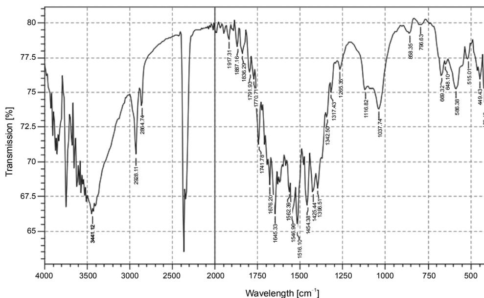
Fig. 3. FTIR spectra of Ag-NPs
