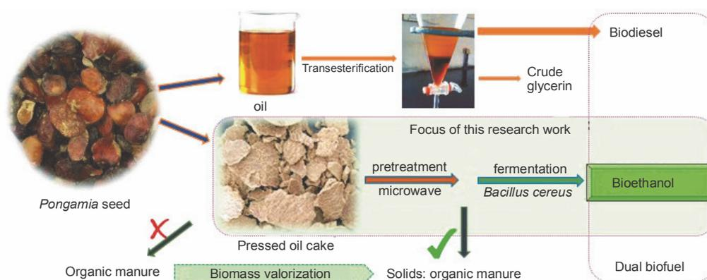
Fig. 1. Scheme of value addition to *Pongamia*-based biofuel production
