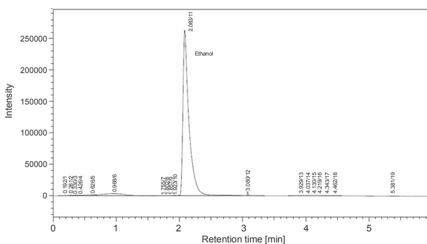
Fig. 2. Gas chromatogram of fermentation distillate showing an ethanol peak
