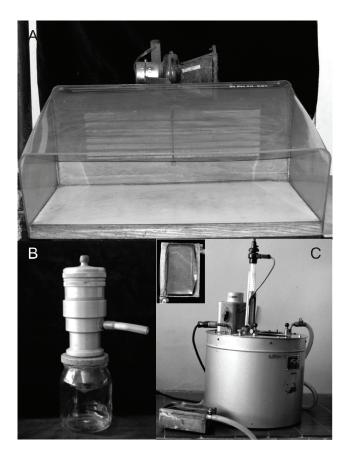
**Fig. 1.** A) A chamber with laminar airflow constructed by E. Pojnar; B) A device for enzyme filtration constructed by E. Pojnar; C) A device attached to a water bath constructed by E. Pojnar
